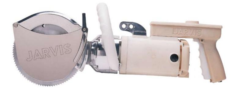
The Jarvis Model SEC 180 electrically powered circular breaking saw.
