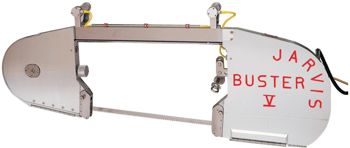
**The Jarvis Model Buster V Loin Drop - electrically powered bandsaw for beef loin dropping (quartering).**
