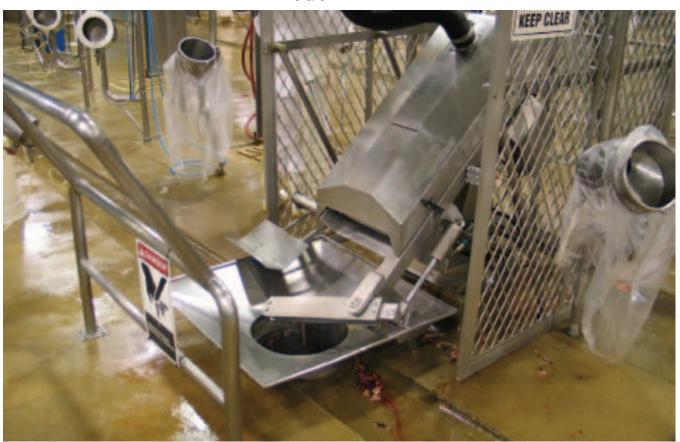
The Jarvis Model AHD-1 Automatic Head Dropper -for continuous sheep head dropping operations on the kill floor.
